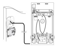
Feed the cable through the slot and then, being careful not to overlap it, zig-zag any excess cable behind the battery pack.
