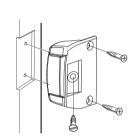
Close the door and using the lock case as a guide mark the position of the remaining component – the 'staple' – on the door frame. Chisel out a recess in the door frame to hold the staple flush with the frame and fix it with the screws provided.
