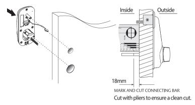
Place the electronic keypad in the hole on the outside of the door.
