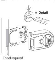
\* If you have used a handing plate on STEP 1-(L) or 1-(R), please turn the follower to the end position according to your direction before fixing the lock case.
