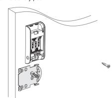
Fix screw to completely secure battery pack.
