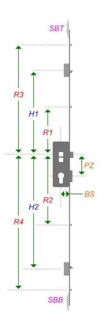
**PZ** – distance from the center of the spindle to the center of the key hole.
